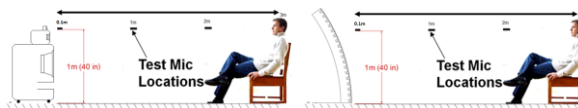
Fig. 14. Illustration of test mic locations for a seated listener at an ear height of 1 m for both systems. Left: conventional system. Right: CBT line array system. The mic locations spanned a distance of 3 m with four locations from 0.1 m to 3 m in steps of 1 m. The first location was very close to the front of each system at 0.1 m!
