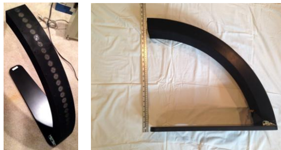
Fig. 32. The 90° ground-plane CBT test array which contains 28 small headphone transducers. The CBT Legendre shading is implemented with a five-bank network.
