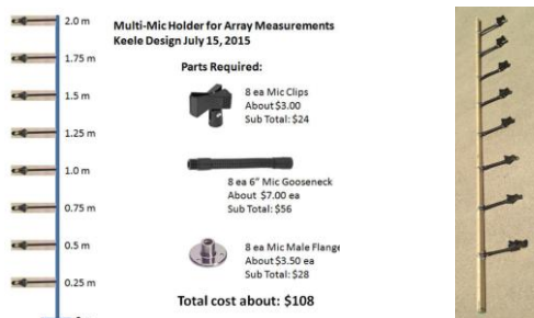
Fig. 35. Multi-mic test jig: plans (left), photo (right). This contraption when attached to a mic stand allows quick movement of the test mic to be positioned at different heights.
